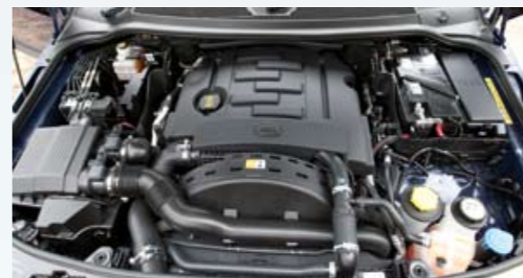
Covers off. Note the lack of room top-left in the D4. The D3 has an ARB compressor added.
