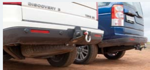
The new Land Rover towbar vs the Mitch Hitch.
